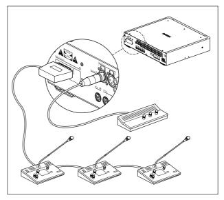
Figure 3.1 Connecting one or more LBB 3222/04 interpreter desks directly to the modular IR transmitter
